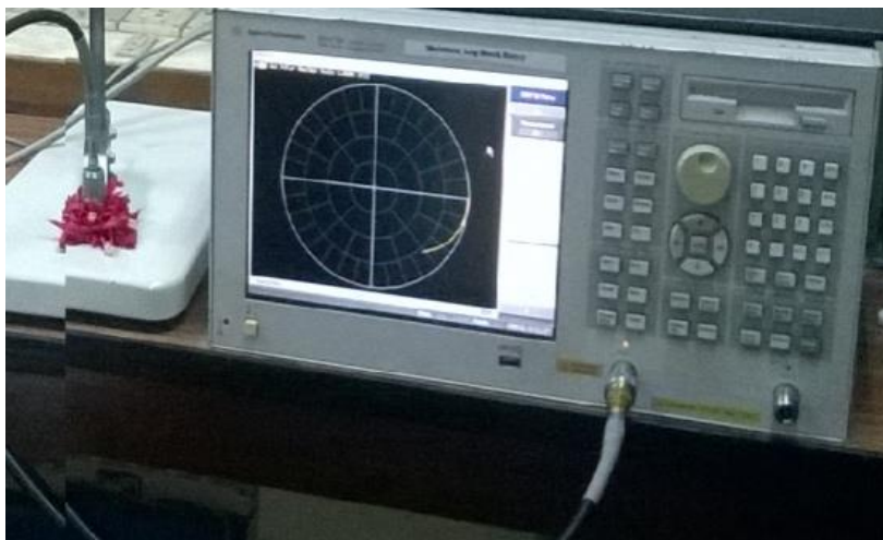
Figure 2: Keywords-Dielectric Properties Flower (Hibiscus), Loss factor, Open ended coaxial probe technique, Permittivity
